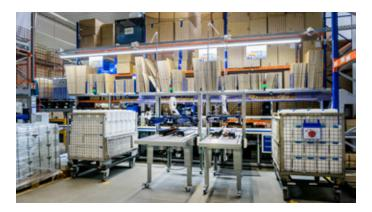
An added value to the new solution, the customer's existing box sealing machines are integrated into the new concept. Two mobile COMFORT.PACK stations with PAPERbubble® paper cushions and AIRplus® air cushions, which are removed from a drawer with a brush system in the table top, were installed for maximum flexibility.
